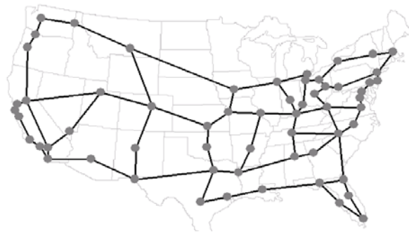
Fig. 3. A typical US backbone network, with 60 nodes and an average nodal degree of 2.6.
